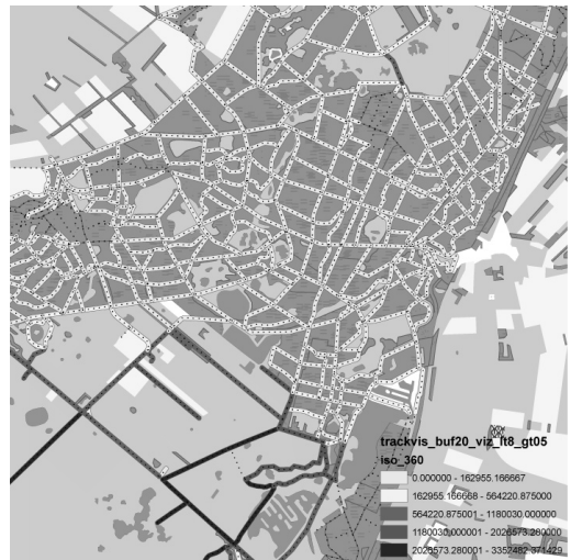
Fig 2: Part of the dataset showing the openness of the landscape based on the visible areas (m2) from a path (calculated at a 50 mtr. Interval)
