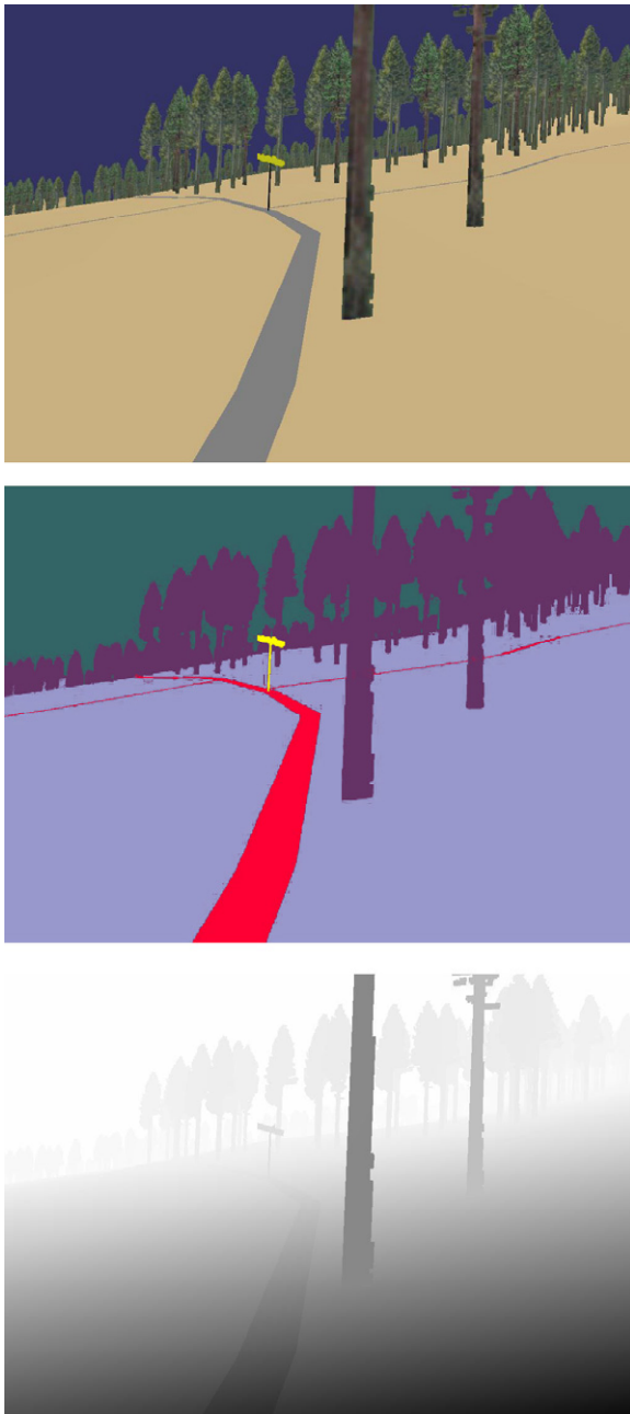
Figure 2. Images rendered by the visibility module. Uppermost image is “true” colour for previewing/presentation purposes; middle image is the false colour, with different colours assigned to different groups; bottom image is the depth image (darkest colour is closest to viewer). The bottom two images are analyzed by the visibility module.
