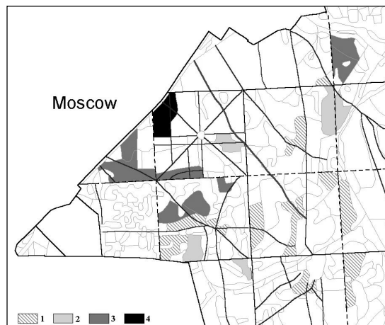
Figure 3. Soil compaction, kg/cm 2 : (1) 1.0-2.0, (2) 2.0-2.5, (3) 2.5-3.0, and (4) >3.0
